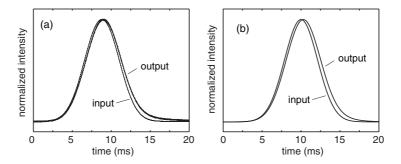
**Figure 5.** Experimental (a) and theoretical (b) input and output pulse shapes for a Gaussian input pulse of 5 ms width (FWHM) after propagation through 4.25 cm of ruby. The output pulse is seen to be delayed and to suffer some distortion.
