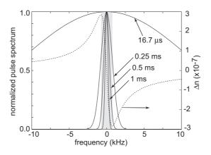
**Figure 3.** Spectra of the input pulses (solid lines) for some of the different pulse widths shown in figure 2, and the change in group index ( $\Delta n$ ) induced by the strong pump beam (dashed line). The grey region shows the range of large anomalous dispersion.
