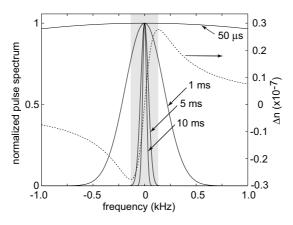
**Figure 7.** Spectra of the input pulses (solid lines) for some of the pulse widths shown in figure 6, and the change in group index  $(\Delta n)$  induced by the strong pump beam (dashed line). The grey region shows the region of large normal dispersion.
