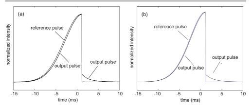
**Figure 8.** Measured (a) and calculated (b) input and normalized output intensities of a truncated Gaussian pulse after propagation through ruby. Without the sharp cutoff, the pulse would have had a width (FWHM) of 10 ms. Note that while the slowly varying leading edge of the pulse experiences a measurable pulse delay, the abrupt trailing edge does not. Thus the front velocity is not equal to the group velocity.
