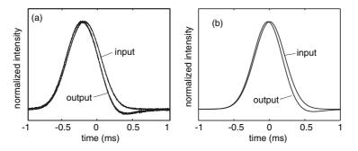
**Figure 1.** Experimental (a) and theoretical (b) input and output pulse shapes for a Gaussian input pulse of 0.5 ms width (FWHM) for propagation through 4 cm of alexandrite. The output pulse is seen to be advanced and to suffer some distortion.
