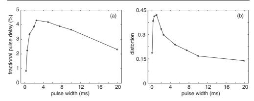
**Figure 6.** (a) Fractional delay of the peak of a Gaussian pulse as a function of pulse width (FWHM) upon propagation through ruby. (b) The distortion (as defined in equation (11)) experienced by the pulse as a function of pulse width.
