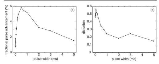
**Figure 2.** (a) Fractional advancement of the peak of a Gaussian pulse as a function of pulse width (FWHM) upon propagation through alexandrite. (b) The distortion (as defined in equation (11)) experienced by the pulse as a function of pulse width.
