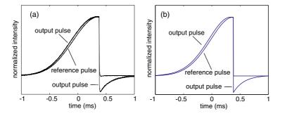
**Figure 4.** Measured (a) and calculated (b) input and normalized output intensities of a truncated Gaussian pulse after propagation through alexandrite. Without the sharp cutoff, the pulse would have had a width (FWHM) of 1 ms. Note that while the slowly varying leading edge of the pulse experiences a measurable pulse advancement, the abrupt trailing edge does not. Thus the velocity of the sharp edge is not equal to the group velocity.
